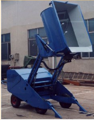
Mixing container can be cleaned or emptied at desired height.
